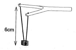
In one test, the elastic band was pulled downwards 6 cm. When released the wooden projectile of mass 20 grammes rose 1.25 m vertically above the catapult. (Air resistance was negligable)
