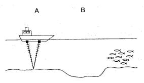
The pulses are short bursts of 40 kHz sound. They are sent at 0.5 s intervals. A screen on board the boat displays the transmitted (T) and reflected (R) signals. The diagram below shows what was seen on the screen when the boat was at position A.
